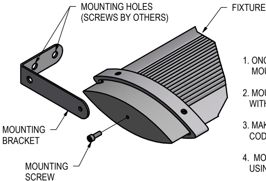
1. ONCE YOU HAVE DIMENSIONS, REMOVE THE MOUNTING BRACKETS FROM THE FIXTURE.
